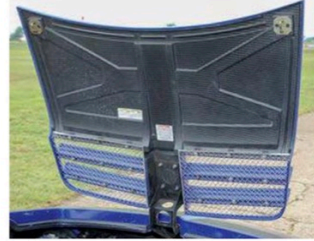
ABOVE: Lightweight, and rather complex, bonnet provides venting for the SV-R's large alloy radiator.
