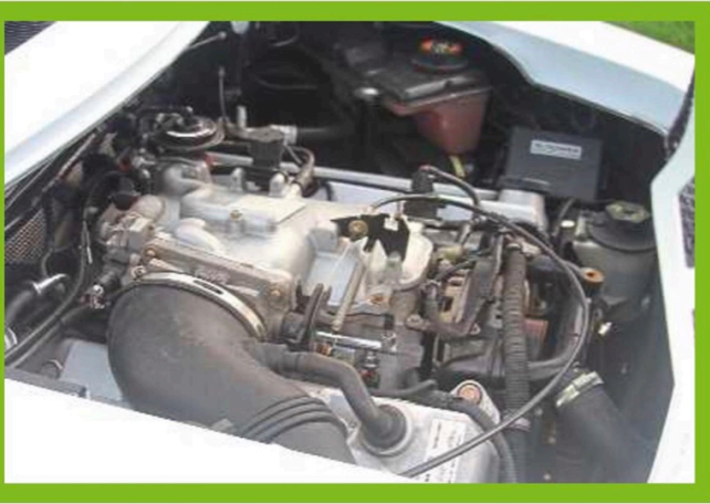
BELOW: A 4.6-litre, quad cam, 32 valve Ford V8 producing 324Ps at 6000rpm and 302lb.ft at 4750rpm powers the SV.
