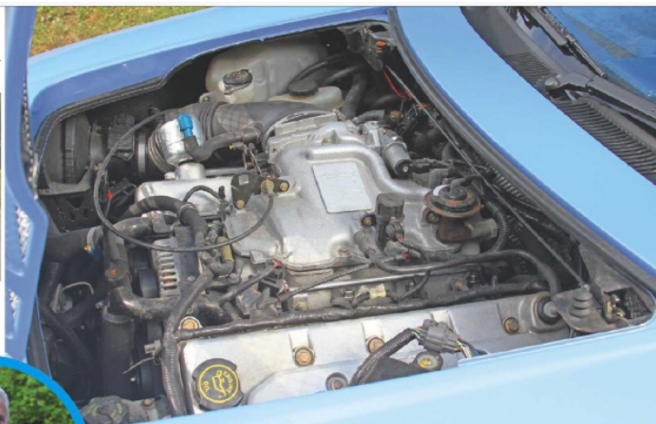
ABOVE: The SV had a 4.6-litre Ford V8. This was enlarged to 5-litres and tuned from 320 to 400Ps for the SVR, though a supercharged SVS with similar power from the smaller engine was ready for 2005.
